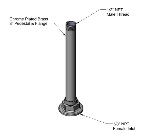
Drawn Checked Approved Product Specifications: **JRM GEF** B-1220 8" Pedestal & Flange Assembly **JHB** Date: Scale: 1:2 04/15/10
