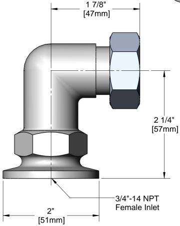
Drawn Checked Approved **Product Specifications: ARH** DMH **JHB** 3/4" NPT Female Inlet 90° Flange, Chrome Polished Brass Date: Scale: 1:1 04/21/09
