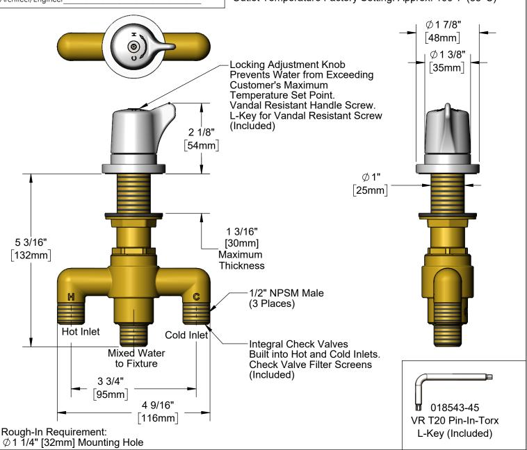
Product Specifications: Above Deck Thermostatic Mixing Valve with 1/2" NPSM Male Fittings Product Compliance:
