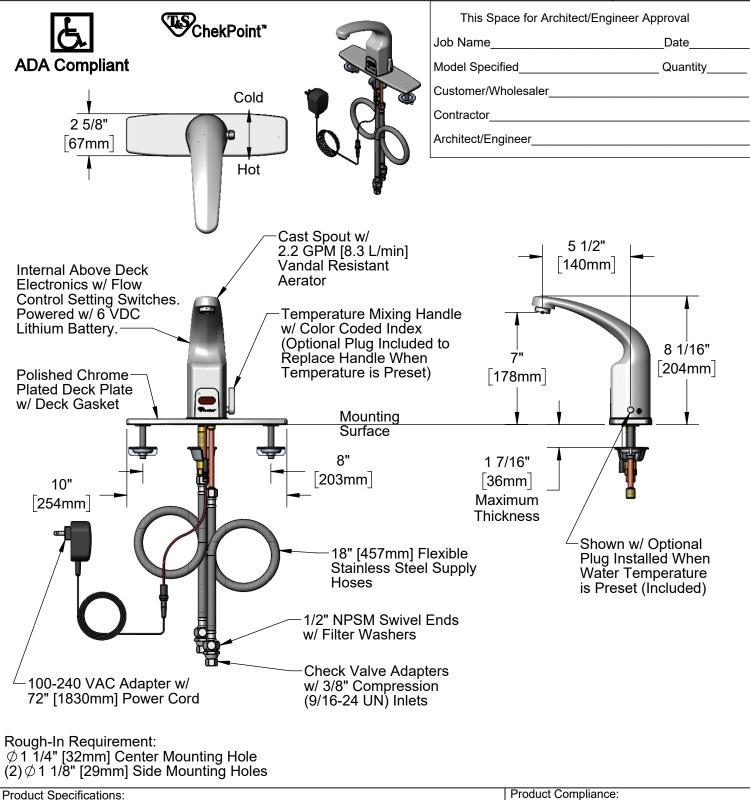
Chrome Plated Brass Above Deck Electronics Faucet, Deck Mount, 8" c/c Deck Plate, Integral Cast Spout w/ 2.2 GPM VR Aerator, Point-of-Use Temperature Control, Battery or AC Adapter Powered, Stainless Steel Flexible Supply Lines & 3/8" Compression Inlets
