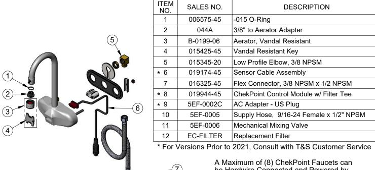
A Maximum of (8) ChekPoint Faucets can be Hardwire Connected and Powered by EC-HARDWIRE ChekPoint Hardwire AC Transformer. (Sold Separately)
