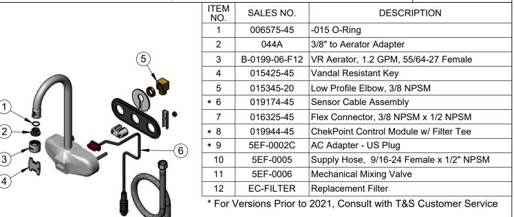
A Maximum of (8) ChekPoint Faucets can be Hardwire Connected and Powered by EC-HARDWIRE ChekPoint Hardwire AC Transformer. (Sold Separately)
