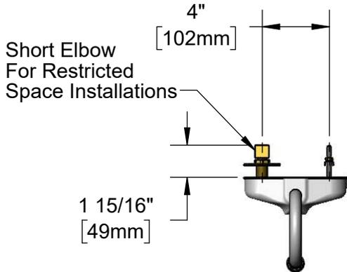
Rigid Gooseneck w/ 2.2 GPM [8.3 L/min] Vandal Resistant Laminar Flow Device
