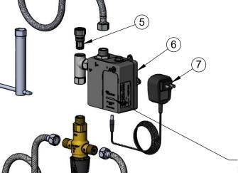
A Maximum of (8) ChekPoint Faucets can be Hardwire Connected and Powered by EC-HARDWIRE ChekPoint Hardwire AĆ Transformer. (Sold Separately)
