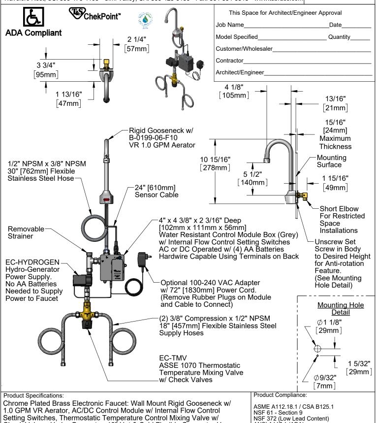
Setting Switches, Thermostatic Temperature Control Mixing Valve w/ Check Valves, Hydro-Generator, 18" Hot & Cold Flexible Connector Hoses
