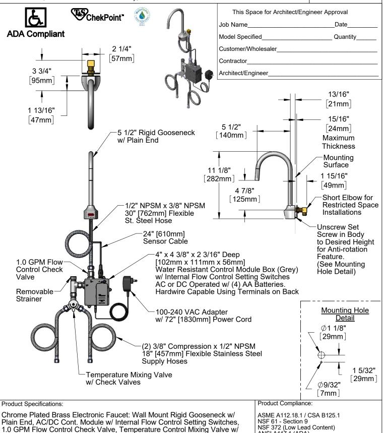
Check Valve, 18" Hot & Cold Supply Stop Flexible Connector Hoses
