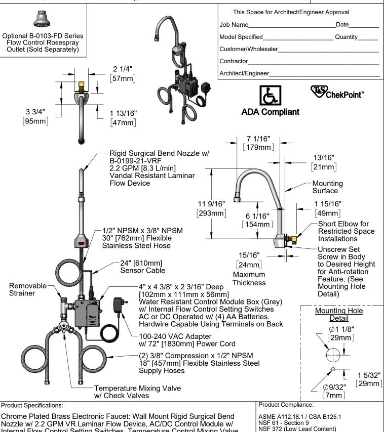
Internal Flow Control Setting Switches, Temperature Control Mixing Valve
