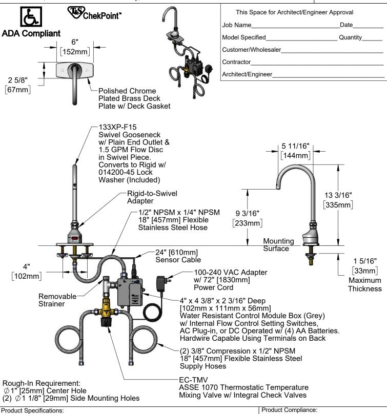
Chrome Plated Brass Electronic Faucet: Single Hole Deck Mount Swivel Gooseneck w/ Plain End Outlet, 1.5 GPM Flow Disc in Swivel Piece, Rigid-to-Swivel Adapter, Deck Plate, AC/DC Control Module w/ Internal Flow Control Setting Switches, Thermostatic Temperature Control Mixing Valve w/ Integral Check Valves & 18" Flexible Stainless Steel Supply Hoses
