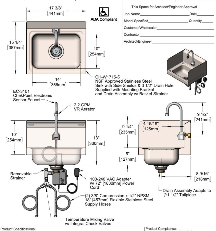
Hand Wash Sink / Elec. Sensor Faucet, Stainless Steel Sink / Backsplash, Side Splash Shields, 3 1/2" Drain Assembly, EC-3101 ChekPoint Electronic Sensor Faucet, Rigid GN w/ VR Aerator, AC/DC Control Module, Temp. Control Mixing Valve, 18" Flexible Supply Hoses
