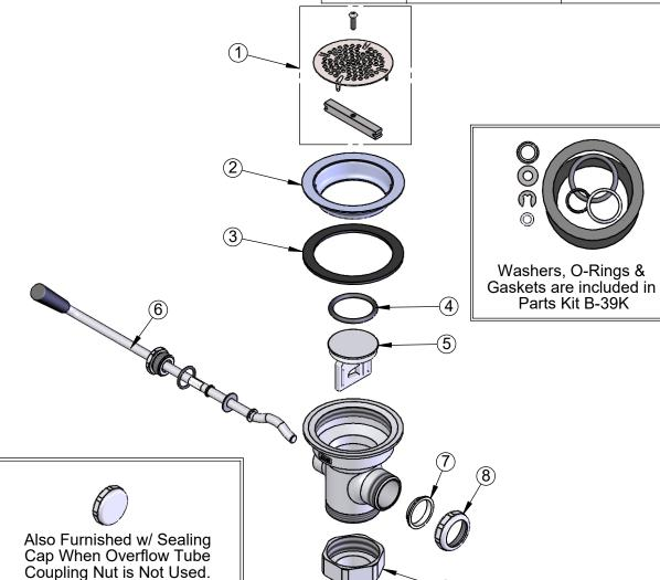
Rotary Waste Valve w/ Twist Handle, 3 1/2" Sink Opening, 2" NPT Male Outlet, 1 1/2" NPT Male Adapter, & Vandal Resistant Flat Strainer
