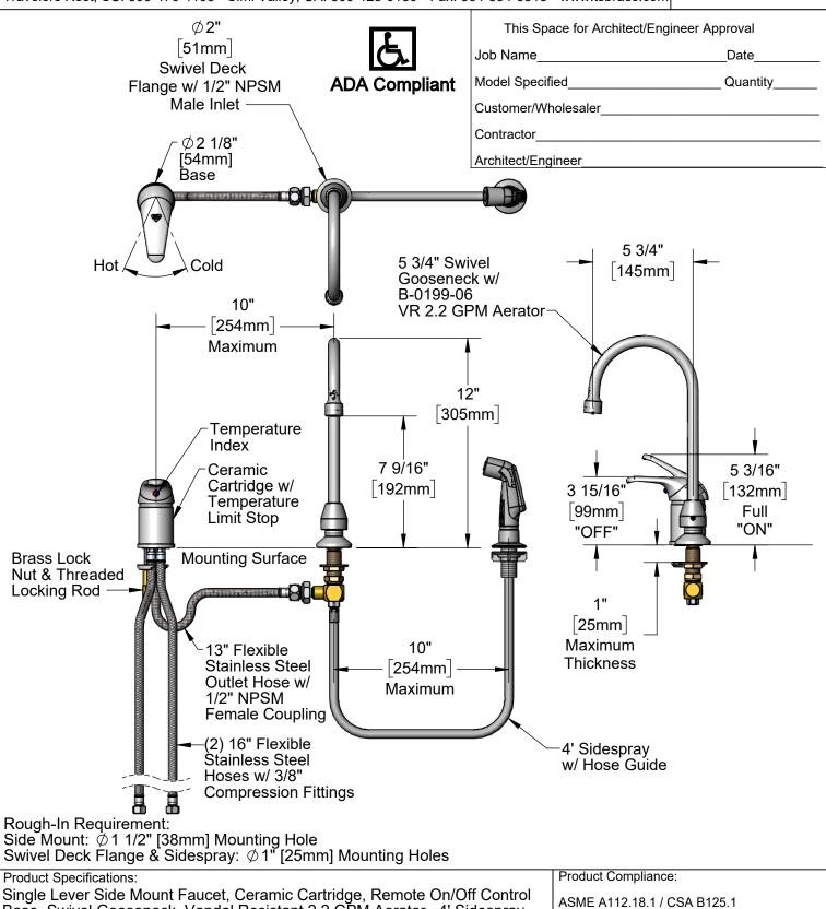
Base, Swivel Gooseneck, Vandal Resistant 2.2 GPM Aerator, 4' Sidespray
