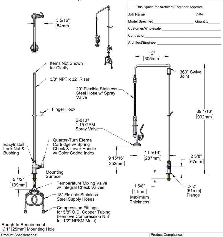
Single Hole, Single Temperature Deck Mount Mixing Faucet, Quarter-Turn Eterna Cartridge w/ Spring Check, Lever Handle, 12" Overhead Swivel Arm, 20" Flexible Stainless Steel Hose, 1.15 GPM Spray Valve, Temperature Control Mixing Valve w/ Integral Check Valves & 18" Flexible Stainless Steel Supply Hoses w/ 1/2" NPSM Male Inlets
