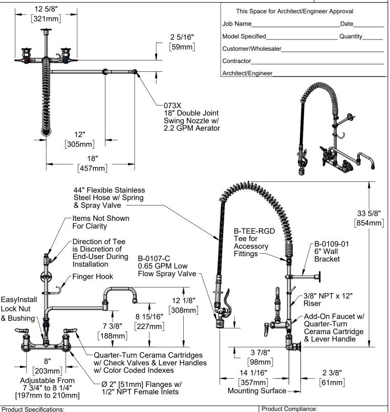
Pre-Rinse Unit: EasyInstall 8" Wall Mount Mixing Faucet, Quarter-Turn Cerama Cartridges w/ Check Valves, Lever Handles, EasyInstall Add-On Faucet, 18" Double Joint Swing Nozzle w/ 2.2 GPM Aerator, 44" Flexible Stainless Steel Hose, 0.65 Low Flow Spray Valve, 6" Wall Bracket, Accessory Fitting Tee & 1/2" NPT Female Inlets
