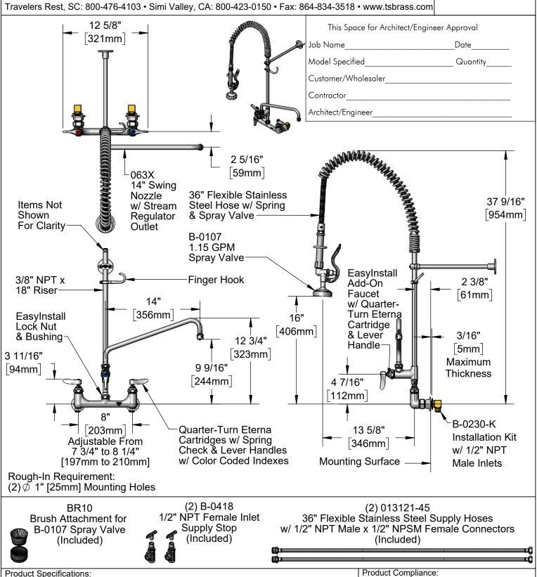
Pre-Rinse Unit: EasyInstall 8" Wall Mount Mixing Faucet, Quarter-Turn Eterna Cartridges w/ Spring Checks, Lever Handles, Add-On Faucet, 14" Swing Nozzle, 36" Flexible Stainless Steel Hose, 1.15 GPM Spray Valve w/ Brush Attachment, Installation Kits w/ 1/2" NPT Male Inlets, (2) 36" Flexible Stainless Steel Hoses & (2) 1/2" NPT Female Supply Stops
