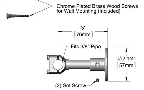
**Product Specifications:** 3" Wall Bracket Assembly for 3/8" Pipe w/ Mounting Hardware
