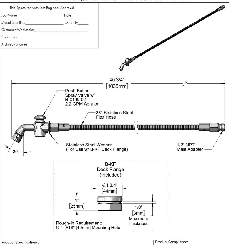
Push-Button Spray Valve w/ 2.2 GPM Aerator Outlet, 36" Stainless Steel Flex Hose & B-KF Deck Flange
