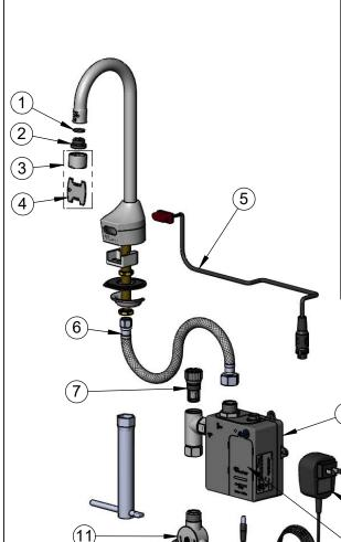
ITEM SALES NO. **DESCRIPTION** NO. 1 006575-45 O-Ring 2 044A 3/8" to Aerator Adapter 3 B-0199-21-VRF VR Device, 2.2 GPM, Laminar Flow, 55/64-27 4 015425-45 Vandal Resistant Key 5 019174-45 Sensor Cable Assembly 6 016297-45 Inlet Hose, Faucet, 1/2" NPSM-F x 1/4" NPSM-F 7 **EC-FILTER** Replacement Filter 8 ChekPoint Control Moudle w/ Filter Tee 019944-45 9 5EF-0002C AC Adapter - US Plug 10 5EF-0005 Supply Hose, 9/16-24 Female x 1/2" NPSM 11 5EF-0006 Temperature Mixng Valve
