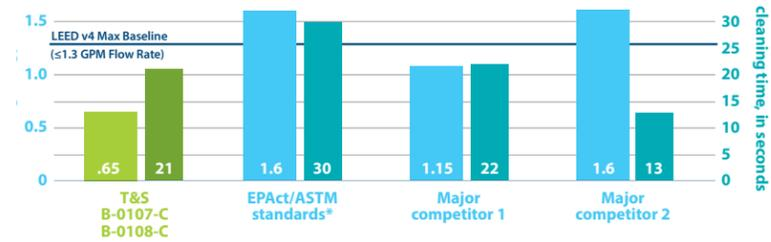
\* The Energy Policy Act of 2005 (or EPA/ASTM) states that all pre-rinse spray valves used for warewashing must have flow rates of 1.6 GPM or lower, while ASTM F2324 states that all pre-rinse spray valves should pass a standardized cleanability test in 30 seconds or less.
